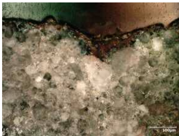
Fig. SF.14. CJ3236 XPL micrograph; detail of the red slag layer (Scale = 500 μm).
