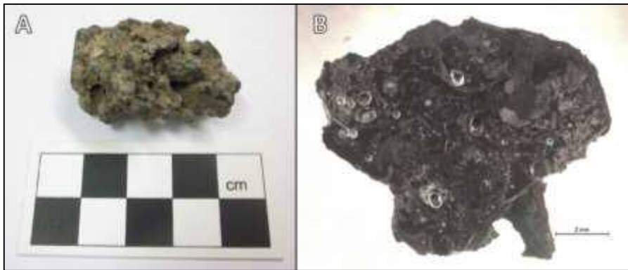
Fig. SF.27. CH4403(10) before sampling (A, note that it had been sampled before by someone else), and in a resin block (B) (Scale in B = 2 mm).
