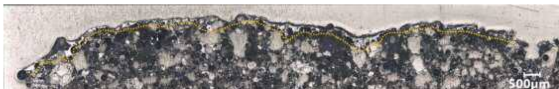
Fig. SF.13. CJ3236 PPL micrograph; inner surface of the crucible with a thin slag layer on its top delimited by the dotted line (Scale = 500 µm).
