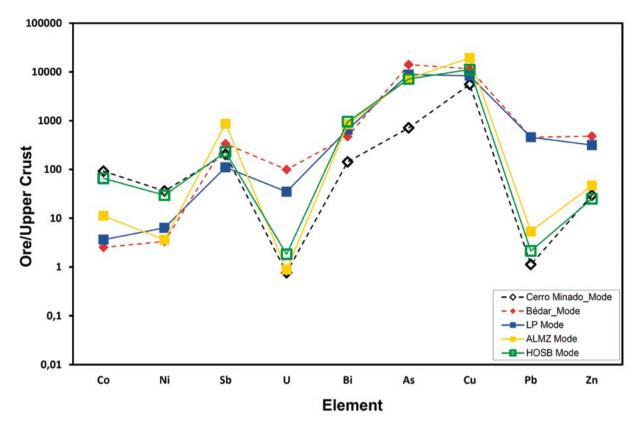
Fig. 7. Normalised multi-element diagram showing patterns in ores from Las Pilas (LP), Almizaraque (ALMZ) and Santa Bárbara (HOSB) in comparison to the patterns shown by the copper mineralisatios of the Vera Basin (Cerro Minado and Pinar de Bédar). Element concentrations normalised to the recommended composition of the upper continental crust in Rudnick and Gao 2014. Geological data from Murillo-Barroso *et al.* 2019 (in colour in the electronic version).
